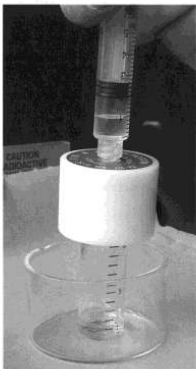
Figure 6 - Isotope Generator during an elution. (The source should be gripped in the operator's other hand for greater stability.)
