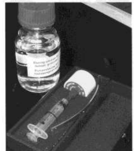
Figure 5 - Isotope Generator in storage box with syringe and tubing. The eluant is in the bottle alongside.
