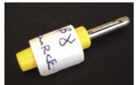
Figure 2 - Irwin diffusion cloud-chamber source. This is the worst example we have met with of an unmarked source. Irwin had drilled into the tip of a 4 mm plug and filled the hole with what we think is a radium-based paint.
