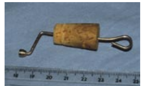
Figure 1 - Griffin diffusion cloud-chamber source. There is radium-based radioluminescent paint on the bell-end of the source holder.
