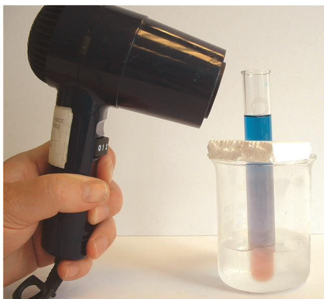
Figure 2 - Using hairdryer used to heat upper half of test tube
