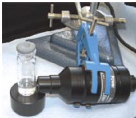
Figure 7 - Monitoring count rate from eluate.
