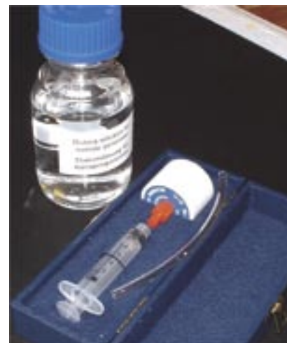
Figure 5 - Isotope Generator in storage box with syringe and tubing. The eluant is in the bottle alongside.
