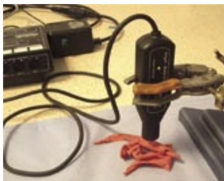
Figure 9 - Monitoring the count rate from balloon fragments.
