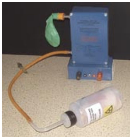
Figure 2 - The Cooknell Ionisation Chamber. The bottle, chamber and balloon form a closed system; when the bottle is squeezed, air is displaced to inflate the balloon, enriching air in the ionisation chamber with thoron gas ( 220 Rn).
