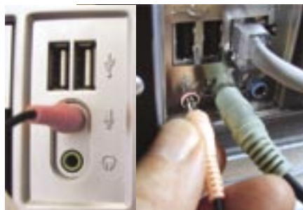
Figures 3a & 3b - Mic inputs (front & rear)
