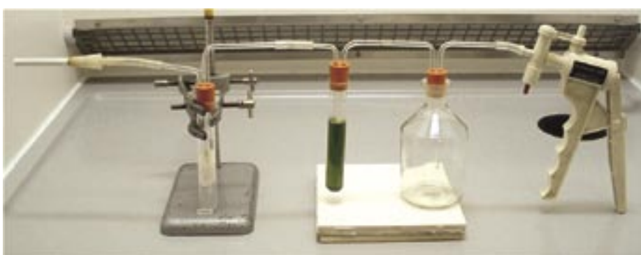
Figure 2 - Puffing model driven by a hand-operated vacuum pump
