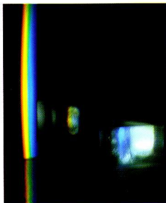
Figure 2 Ribbon spectrum created with 40° x 0.5° LSD set up in the refracted radiation. The LSD's plane is vertical and orthogonal to the radiation.
