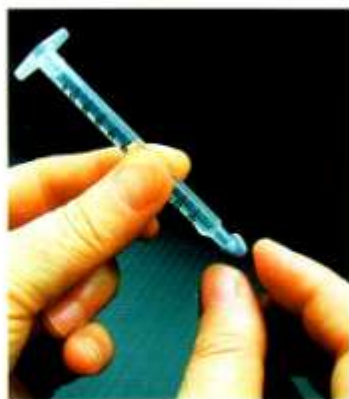
Figure 7 Sealing nozzle with Blu-tak
