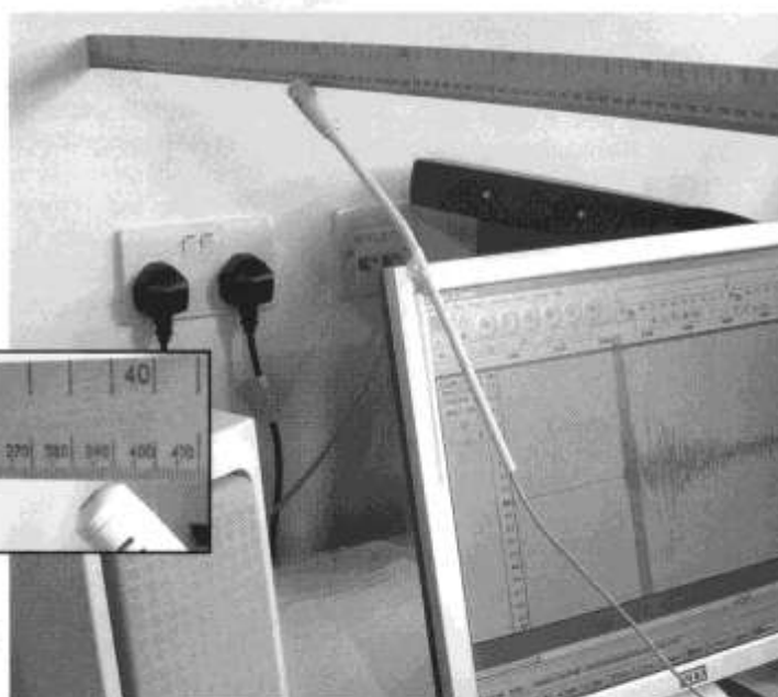
Figure 20 - Measuring distance from the microphone to the wall
