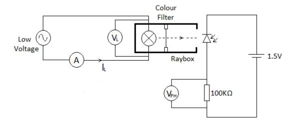
$V_L$ ,  $I_L$  and  $V_{PH}$  are all recorded for a range of raybox voltages from 4V (lamp dim) through to 12V (lamp bright).
