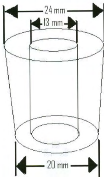
Figure 7 Dimensions for CO 2 sensor adaptor for a boiling tube – made by boring out the centre of a rubber bung.
