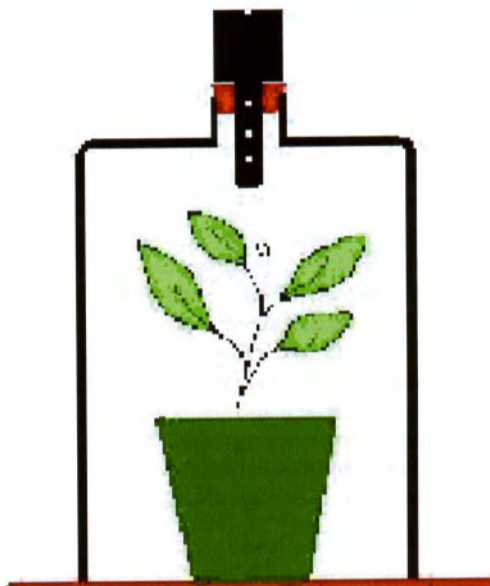
Figure 8 Sensor used with a bell jar on a glass sheet.
