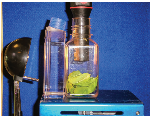
Figure 6 Experimental set-up for measuring respiration and photosynthesis rates in plants. Basil leaves are placed into a 'reaction chamber' together with a \text{CO}_2 gas sensor from Instruments Direct Services Ltd (product code VR105512). The sensor is linked to a computer via a Vernier GoLink interface.
