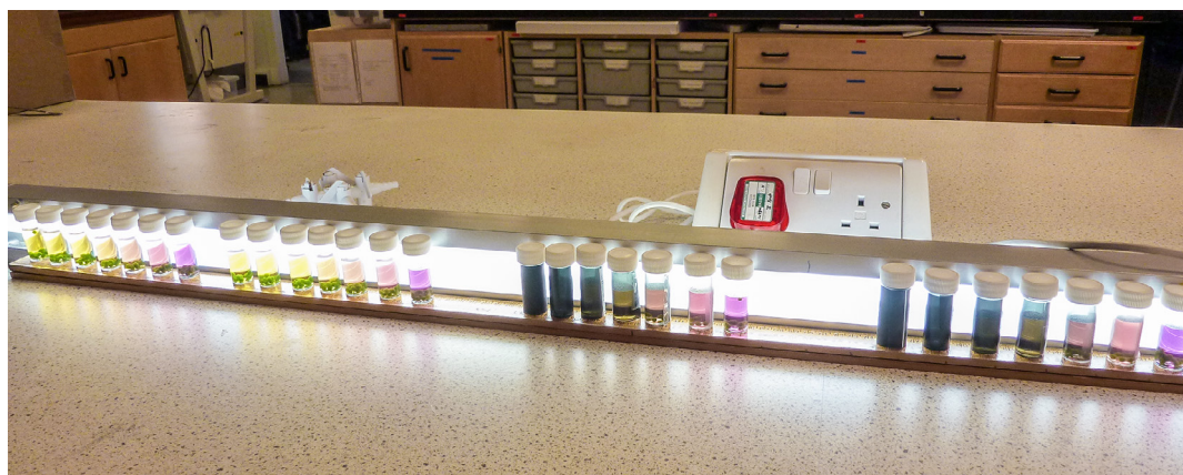
Figure 5 An experimental set-up allowing for measurement of the effects of light intensity on the rate of photosynthesis. Bijou bottles containing immobilised algae are exposed to light from a fluorescent tube; light intensity is altered by the addition of a suitable filter.
