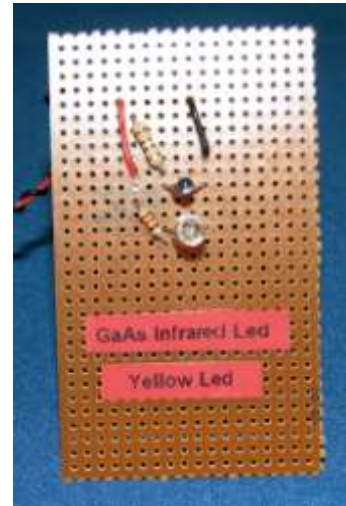
Circuit with yellow and infrared LEDs..
