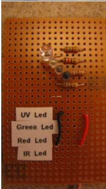
LED array on stripboard.
