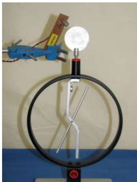
Irradiating the zinc plate on a Frederiksen electroscope, 4410.00
