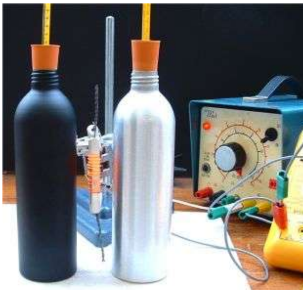
DIY Radiant Heat Source mounted vertically between black and silver cans.
