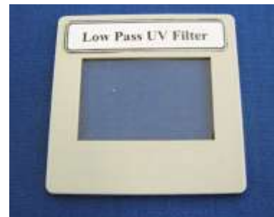
UV Filter cut from sheet supplied by Edmund Optics, NT39-426 and put into a slide mount.
