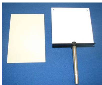
Zinc sulphide screens: Leybold, 468 72 (Left) Frederiksen, 3075.00 (Right)
