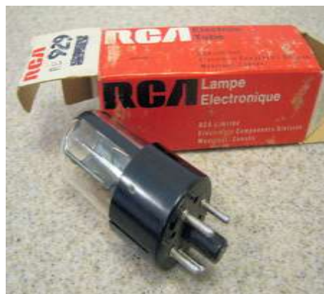
RCA phototube type 929. A strip of black tape masks the anode from light. The curved metal sheet at the back of the tube is the cathode.
