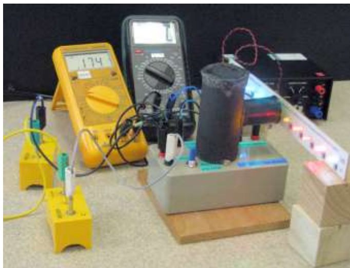
Photo opposite: The phototube is mounted on an octal base on top of the grey box. The tube is screened from ambient light by a T-shaped tubular blackout. The tube is being irradiated with light from one LED on the array of LEDs.
