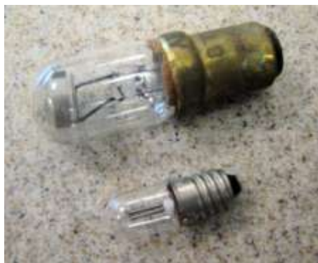
Two neon lamps, electrodes showing. TOP: SBC base, ring and disc electrodes. BOTTOM: MES base, rod electrodes.
