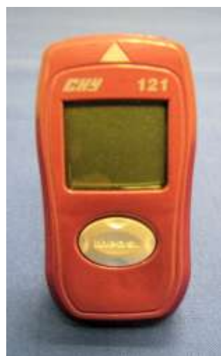
Non-contact temperature sensor: SEP (161-300).
