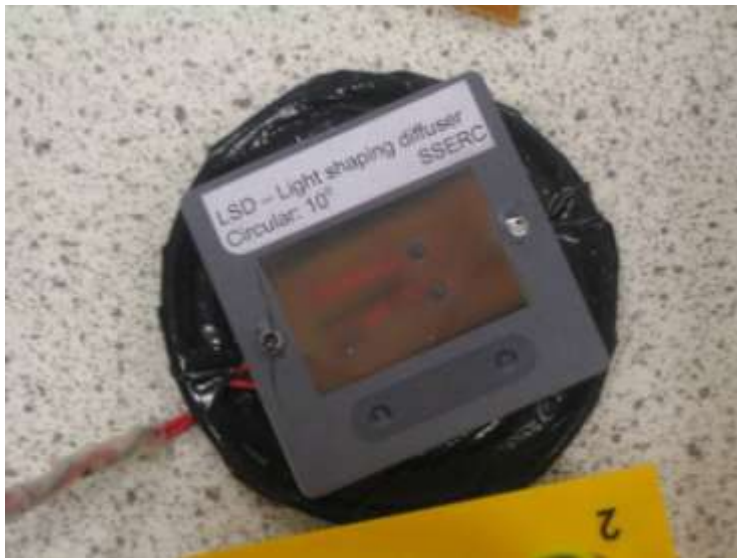
Two LEDs mounted 6 mm apart behind light-shaping diffuser on canister lid.
