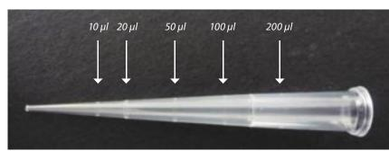
Figure 3 - Syringe tip showing graduation marks.
